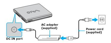
2 Plug the power cord into the AC adapter and an AC outlet.
